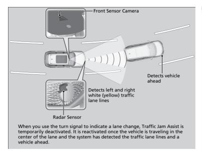
When the driver takes direct control of steering, the steering assist function is temporarily canceled.
