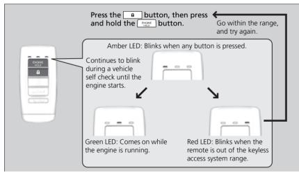
The engine runs for up to 10 minutes without you starting the vehicle. To extend the run time for another 10 minutes during the first run, press the <u>a</u> button, then press and hold the <u>rece</u> button.
