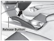
**To apply:** Pull the lever fully up without pressing the release button.
