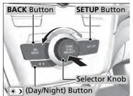
Use the selector knob or **SETUP** button to access some audio functions.
