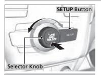
Press the **SETUP** button, and rotate n to select **Sound Settings**, then press s. Rotate n to scroll through the following choices:
