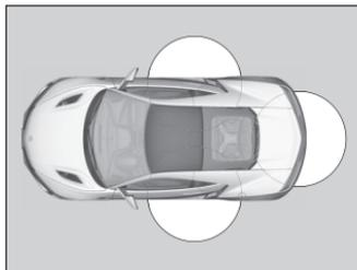
When you carry the keyless access remote, the outer door handles automatically pop in/out and you can lock/unlock the doors and open the hatch.
