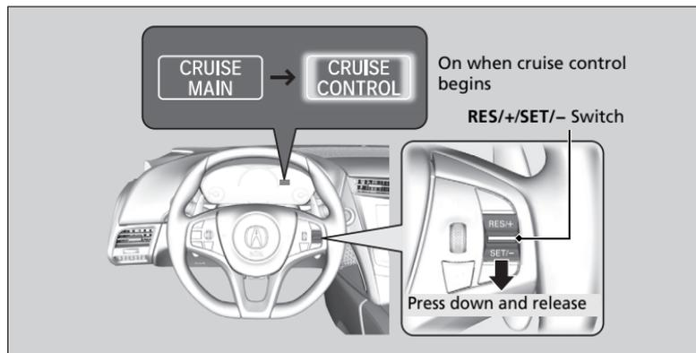
Take your foot off the pedal and press the **RES/+ / SET/-** switch down when you reach the desired speed.
