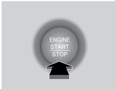
**Note:** The power system is harder to start in cold weather and in thinner air found at altitudes above 8,000 feet (2,400 m). When turning on the power system in cold weather, turn off all electrical accessories such as the lights, climate control system, and rear defogger in order to reduce 12-volt battery drain.
