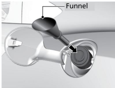
5. Fill the tank with fuel from the portable fuel container. Pour fuel carefully so you do not spill any.
