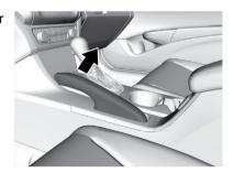
To release: 1. Pull up the lever slightly and press and hold the release button.
