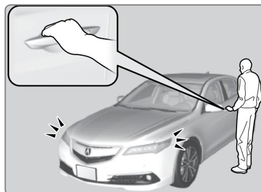
**To lock:** Press the door lock button on either front door (or rear door\*) handle when the vehicle is off. If the remote transmitter is inside the vehicle, the doors will not lock.
