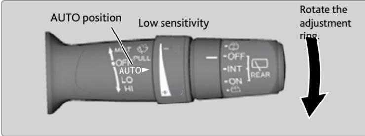
Return the lever to the OFF position when rain stops.
