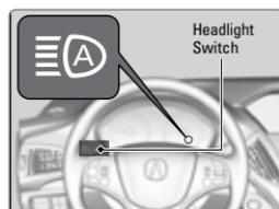
**To disable the system:** When the vehicle is on and parked, pull the headlight lever towards you and hold it for 40 seconds. The auto high-beam indicator blinks twice.
