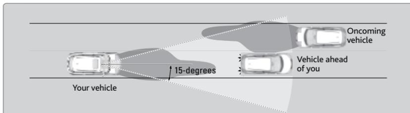
If a vehicle is detected ahead of you, the headlights stay in low beams. If the system does not detect any vehicles ahead of you, the headlights change to high beams.
