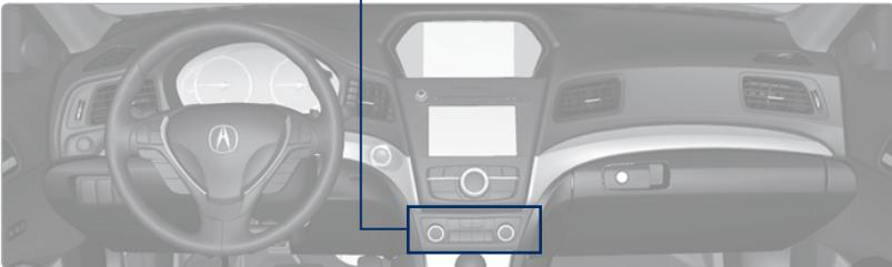
On vehicles with ODMD, climate information is displayed on the screen, but cannot be selected via touch. Adjust the climate settings using the buttons.
