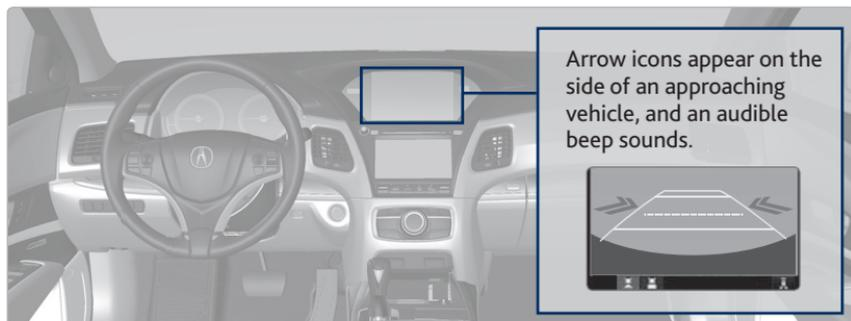
The system does not provide alerts for a vehicle that is moving away from your vehicle, and it may not detect pedestrians, bicycles, or stationary objects.
