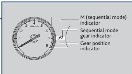
**When D is selected:** The vehicle goes into sequential shift mode momentarily, and the gear indicator comes on. When you start driving at a constant speed, sequential shift mode automatically switches off, and the gear indicator goes off. Hold the (+) paddle shifter for two seconds to return to normal drive.
