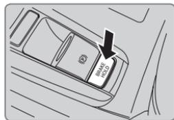
Press the accelerator pedal to cancel brake hold and start moving.
