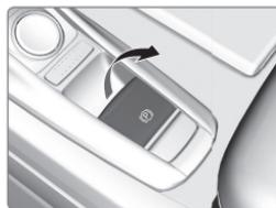
**To release:** Press the brake pedal and make sure your seat belt is fastened. Press the switch down to release.
