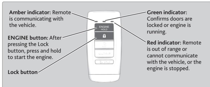
Make sure the vehicle is in a safe location when using remote engine start (i.e., a well ventilated area, away from flammable materials).
