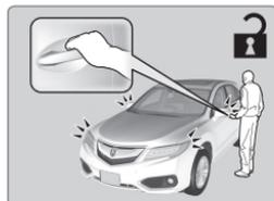
**To lock:** Press the door lock button on either front door handle when the vehicle is off. If the remote transmitter is inside the vehicle, the doors will not lock.
