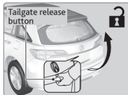
**To lock:** Press the tailgate lock button to lock the tailgate and all doors. If the remote transmitter is inside the vehicle, the tailgate and doors will not lock.
