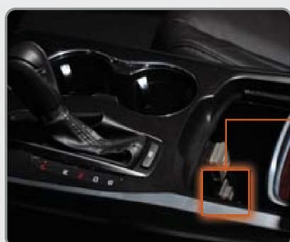
Slide back the center console door to connect a USB flash drive or iPhone/iPod dock connector to the USB port.
