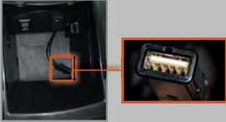
2. **Connect** the USB connector to your iPod dock connector or flash drive.
