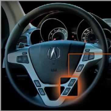
Press the Info button to toggle to the "Keyless Memory Settings" display, then press SEL/RESET to activate the menu.
