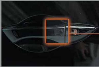
**Press** the door lock button on either front door handle.
