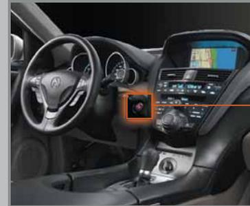
**Press** the ENGINE START/STOP button once.
