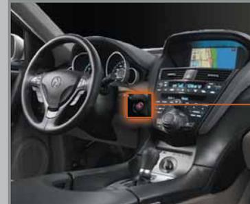
**Press and hold** the brake pedal then **press** the ENGINE START/STOP button.
