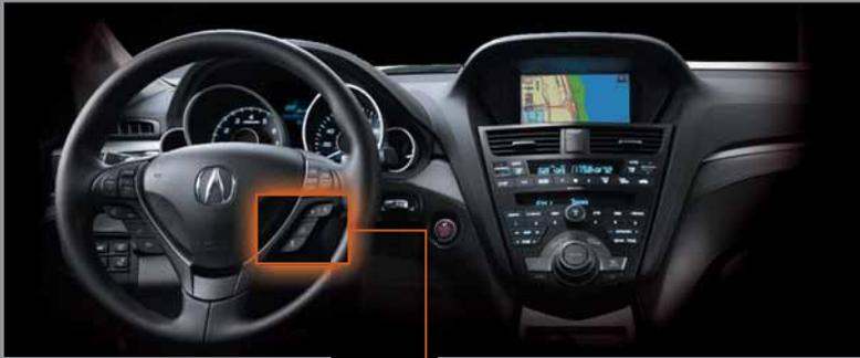
While on the Trip Computer display, **press** the SEL/RESET button to access trip information. **Press** either Info (▲/▼) button to toggle through the various screens, or the SEL/RESET button for sub-displays.
