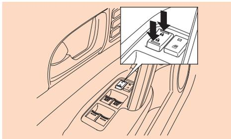
When the driver's door lock tab is pulled back, all doors are locked. Pushing forward on this locking tab unlocks only the driver's door. When any door is unlocked, you can see the red indicator on the lock tab.
