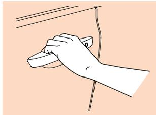
The handle of each front door has a sensor, which works with the remote so you can automatically unlock the door(s).
