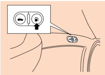
To open the fuel fill door, press the button on the driver's door.
