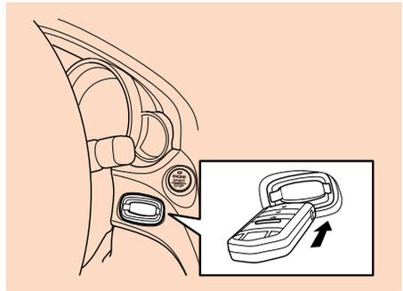
**To use:** Insert the keyless access remote into the slot, with the lock button side (not the side with the built-in key) forward, and push firmly.
