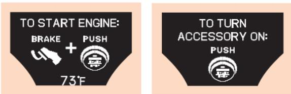
**To start the engine:** Press the brake and push the engine start/stop button. This is called the **On Mode**.
