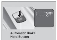
While the system is on, press the automatic brake hold button again.
