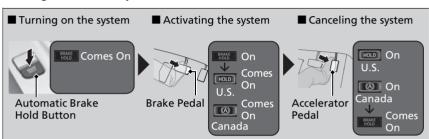
Fasten your seat belt properly, then start the engine. Press the automatic brake hold button.
