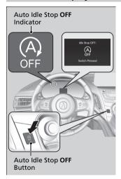
To turn the Auto Idle Stop system off, press this button. The Auto Idle Stop system stops.
