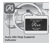
The Auto Idle Stop suspend indicator comes on and a message appears on the multi-information display. When the Auto Idle Stop system cannot be activated.
