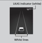
When the LKAS is suspended, green lines on the gauge change to white lines or disappear, and the beeper sounds (if activated).
