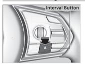
Press the interval button to change the ACC with Low Speed Follow following-interval. Each time you press the button, the following-interval (the interval behind a vehicle detected ahead of you) setting cycles through short, middle, long, and extra long following-intervals.
