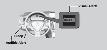
You can change the distance (**Long/Normal/Short**) between vehicles at which the system's earliest collision alert will come on through multi-information display or information screen setting options.
