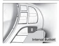
Press the 🖹 (interval) button to change the ACC following-interval. Each time you press the button, the following-interval (the interval behind a vehicle detected ahead of you) setting cycles through extra long, long, middle, and short following-intervals.
