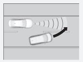
Depress the brake pedal and take direct control of steering.
