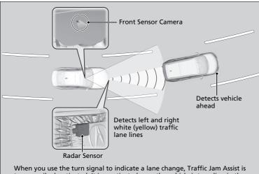
temporarily deactivated. It is reactivated once the vehicle is traveling in the center of the lane and the system has detected the traffic lane lines and a vehicle ahead.
