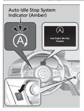
To turn the Auto Idle Stop system off, press this button. The Auto Idle Stop system stops.
