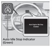
The engine then restarts once the vehicle is about to move again, and the indicator (green) goes off.
