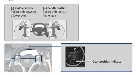
When the transmission is in D: The vehicle goes into sequential mode and the gear selection indicator becomes more prominent. Sequential mode will cancel if you hold the (+) paddle shifter for a few seconds, travel at a constant speed, come to a complete stop, or change to another Integrated Dynamics System (IDS) mode.
