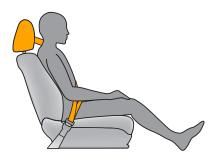
Adjusting a head restraint so the center is level with the back of the occupant's head (or as high as possible for taller people) can help reduce injuries during a rear impact.
