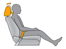
In vehicles equipped with active head restraints, the restraint will move up and forward a little when enough pressure is applied against the seatback.
