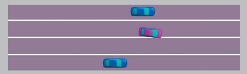
If you cross a detected lane line without using your turn signal, a message appears on the MID and a beep sounds. Steering torque is applied to keep your vehicle in the middle of the lane.
