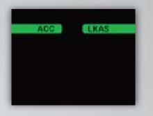
2. Press the LKAS button. Lane outlines appear in the MID. Dotted lane lines turn solid when the system operates.
