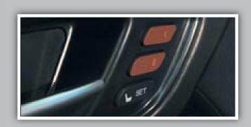
**Note:** Stored positions can also be recalled by pressing one of the memory buttons (1 or 2) on the door.
