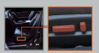
4. **Press** the memory button corresponding to the remote (1 or 2) you are using. You will hear two beeps.
