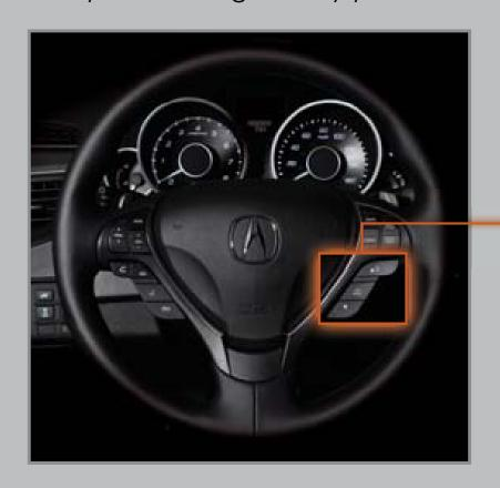
**Press** the Info button to toggle to the Customize Settings display, then **press** SEL/RESET to enter the menu.
