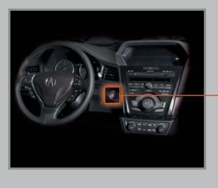
Press ENGINE START/STOP once without pressing the brake pedal for Accessory mode. Press it again for On mode.
