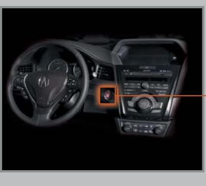
Press and hold the brake pedal, then press ENGINE START/STOP.
