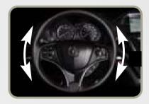
Additionally, a small amount of steering torque is applied to keep your vehicle in the center of the lane. Keep your hands on the steering wheel and steer the vehicle as necessary to remain in the center of the lane.
