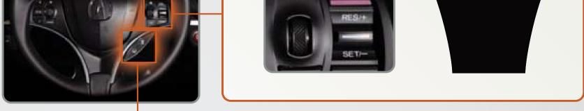
Press the LKAS button. Lane outlines appear in the MID. Dotted lane lines turn solid when the system operates.
