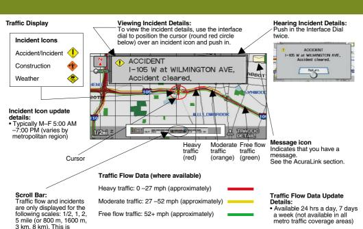
Real-Time Traffic Display: The navigation screen can display up-to-the-minute traffic information when available including flow (traffic speed), accidents, and construction on freeways in major metro areas. The display of traffic flow and incidents on your map screen is optional and can be turned On/Off by selecting the "Traffic" icon on the Icon bar (see the Navigation Owner's Manual for details).
